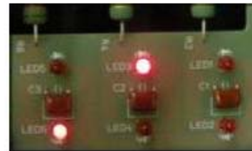
LED indication in compressor protection control
